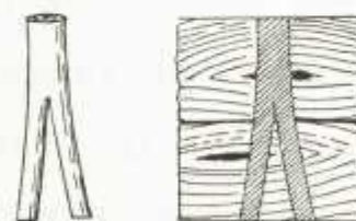
FIGURE 7 FASTENING WITH FORKED PIN FROM A HEAD-REST
